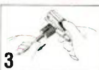
3 Press down lever and pull out cable.
