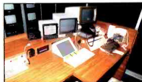
Producer's station, with interface computer terminal at center (countersunk monitor). Two video monitors on overbridge behind the terminal show teleprompter and Betacart status displays, respectively. Terminal at far right is part of original newsroom computer system.
