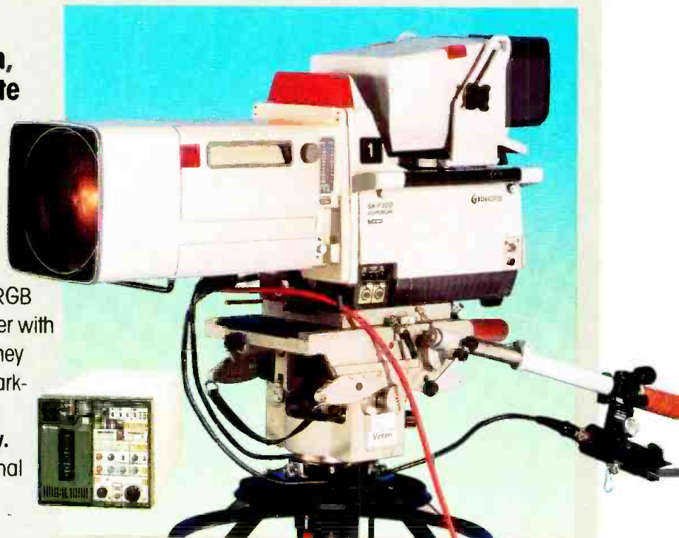
New space-saving 1/2-rack CCU with built-in power supply.
