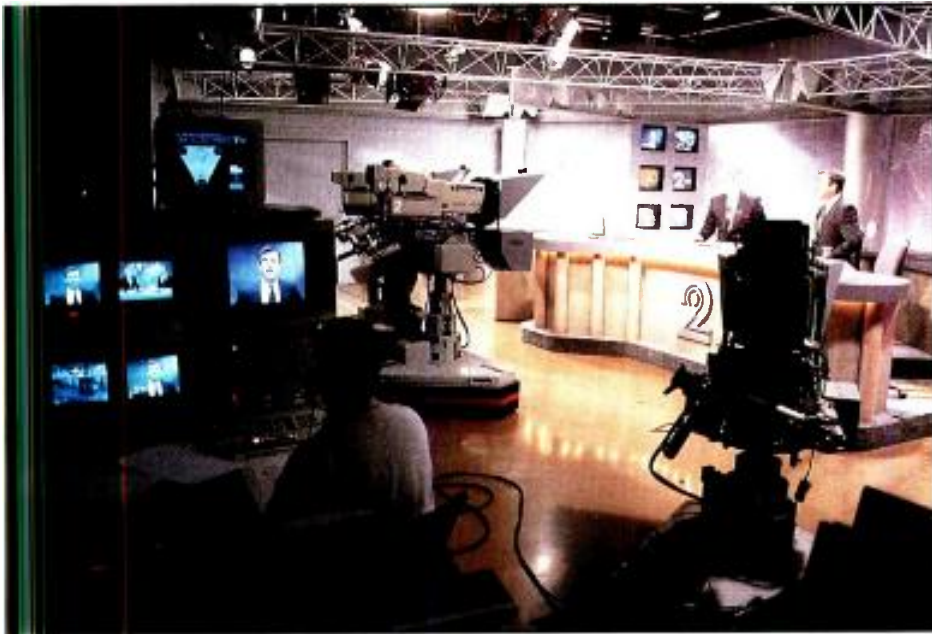
The robotic camera control position in the news studio at Detroit's WJBK-TV controls three fully automated pedestals.
