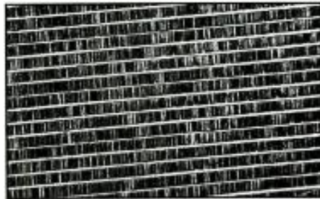
The trend toward increased recording density is clearly visible in these magnetically “developed” micrographs. At left, a 50× magnification of Betacam’s component analog format is shown (darker tracks are C, lighter tracks are Y). At right, the component digital D-1 format is shown at the same magnification. (Courtesy of 3M.)
