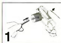
1 Insert end of cable into the stripper.
